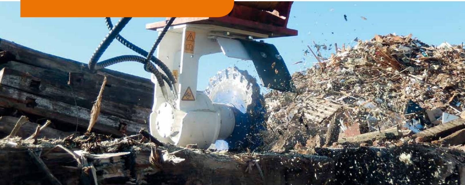
◀ An **ES45HD** cuts quickly and efficiently through large wooden beams.
