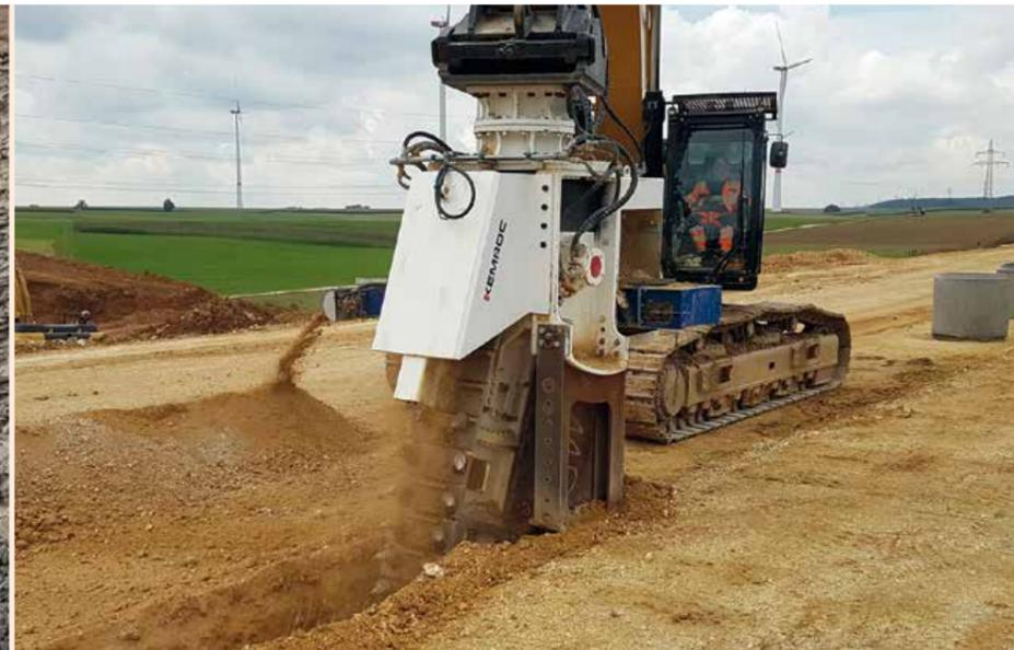
▲ This **ETR3** trencher excavates a 60 cm wide trench with variable depth in a soft limestone with a uniaxial compressive strength of 60 MPa. The trench was cut to the side of the excavator tracks and the cutting speed was 50 m/h.
