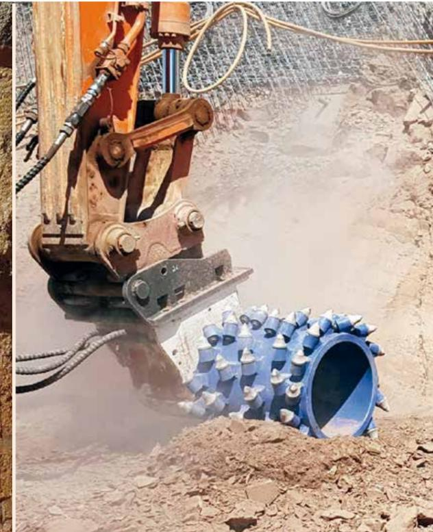
▲ An ideal tool for profiling work; this **ES80HD**, fitted with an 80 cm wide cylindrical cutter drum, is grinding a sandstone embankment.
