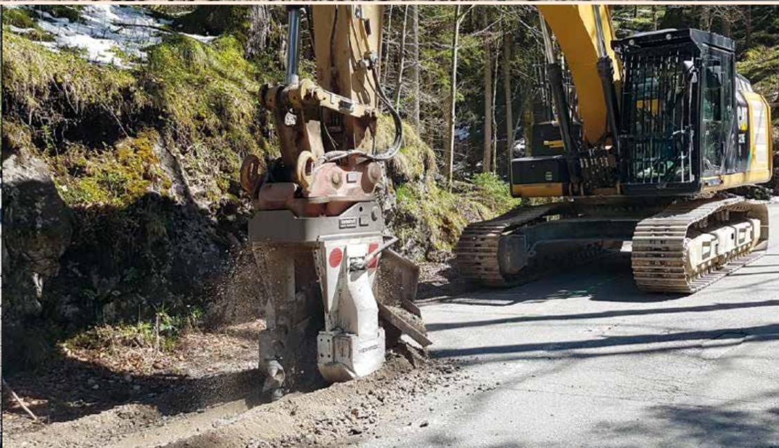
▲ This **EK100** chain cutter excavates a 70 cm wide by 1.2 m deep trench in shale with ease.
