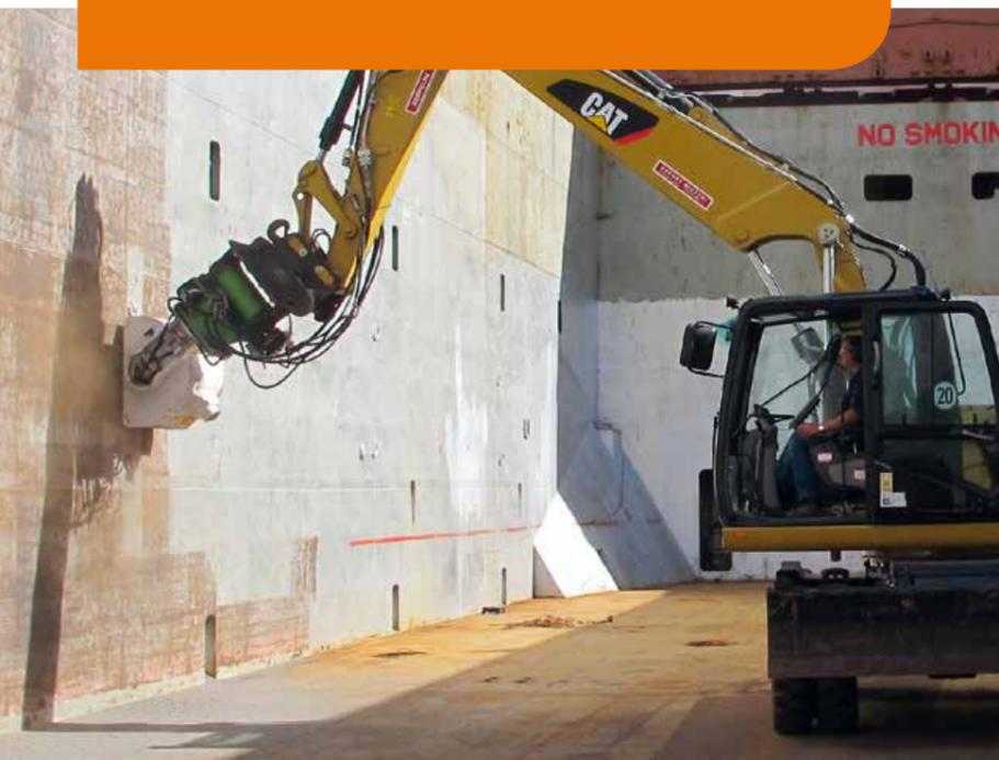
◀ An **EXRUST60** used to remove paint from walls inside the hold of a ship. Approximately 300 m<sup>2</sup> of wall were cleaned per hour!
