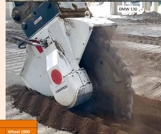
Cutter wheels in the DMW range were designed in cooperation with customers for attachment to hydraulic excavators. Two high torque, lateral hydraulic motors guarantee high production rates and maximum cutting forces. As a result, even in hard rock with a uniaxial compressive strength of 120 MPa as well as reinforced concrete, very high productivity rates can be achieved. KEMROC produces these robust attachments in 4 sizes for excavators from 14 to 60 tons.
