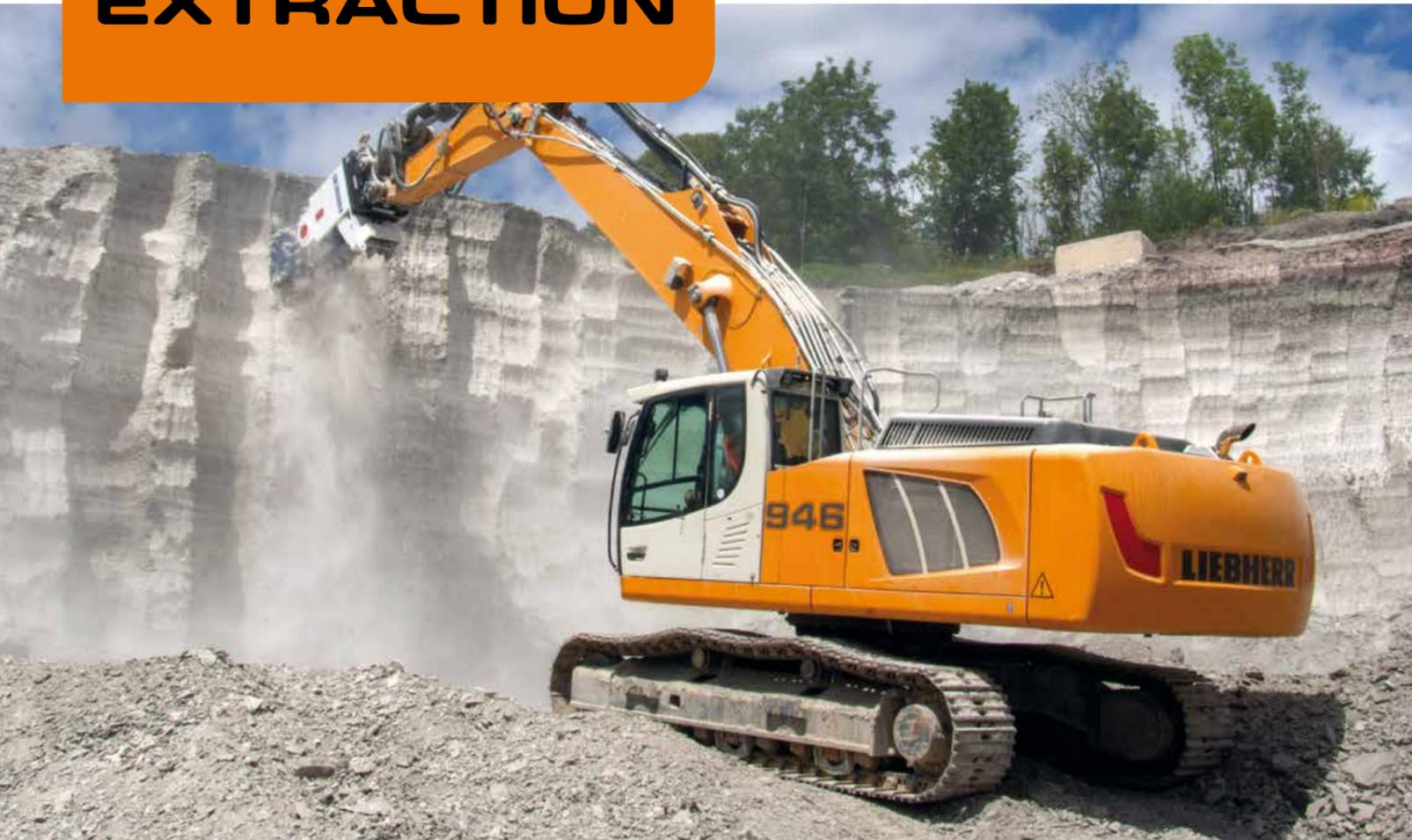
▲ Powerful and efficient gypsum mining with an **EK 140** with 900 mm cutter width mounted on a Liebherr 946. Production rate was approx. 110 tons per hour.
