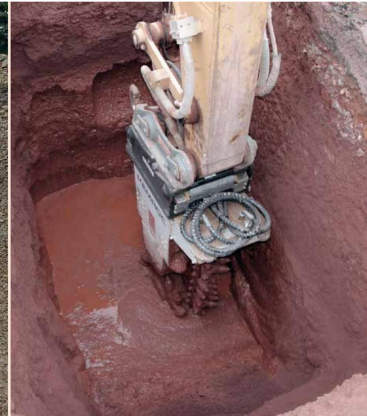
▲ Impressive productivity in narrow trenching. An **EK 100** chain cutter with 700 mm wide cutter head excavates almost 15 m/h of trench. With a central cutter chain, it works effectively without having to swing sideways. This saves energy which can be used for productivity and is kind to the excavator.
