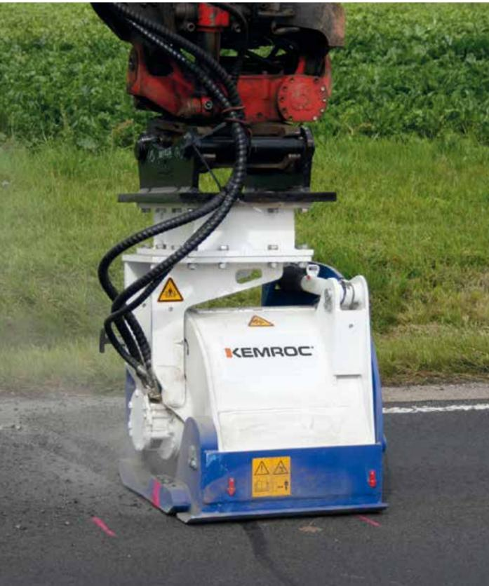
◀ An **EX45HD** planing a 4 cm deep strip from an asphalt surface. The rotation module allows the planer to work in a direction at an angle to the axis of the excavator.
